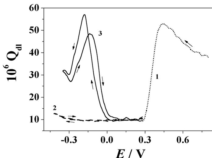
Fig. 5. Double layer pseudocapacitance  $Q_{dl}$  variation with the potential of Au electrode (1) and Au electrode coated with selenium atomic layer (2,3). Electrolytes: 1mM  $SeO_2$  + 0.1M  $HClO_4$  (1), 0.1M  $HClO_4$  (2), 1mM  $Pb(ClO_4)_2$  + 0.1M  $HClO_4$  (3).
