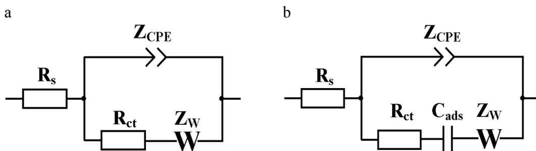
Fig. 2. The best fit equivalent electric circuits for the potentiodynamic frequency response of (a) Se atomic layer deposition on Au and Pb upd on Se atomic underlayer, (b) Pb upd on Au.  $Z_{CPE}$  is the impedance of a constant phase element,  $Z_W$  – impedance of Warburg element,  $R_{ct}$  – charge transfer resistance,  $C_{ads}$  – adsorption capacitance,  $R_s$  – resistance of electrolyte solution.
