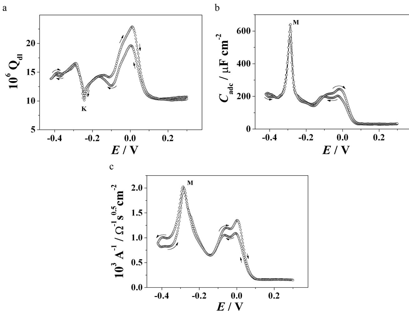
Fig. 4. EEC parameters variation in cyclic potential scan in Pb upd on Au: (a) double layer pseudocapacitance  $Q_{dl}$ , (b) adsorption capacitance  $C_{ads}$ , (c) inverse Warburg constant  $A^{-1}$ .
