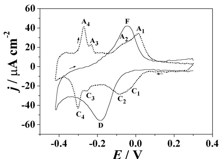
Fig. 3. Cyclic voltammograms of bare Au electrode (dotted) and Au electrode coated with selenium atomic layer (solid) in 1 mM  $Pb(ClO_4)_2$  + 0.1 M  $HClO_4$ .  $dE/dt = 58$  mV/s.
