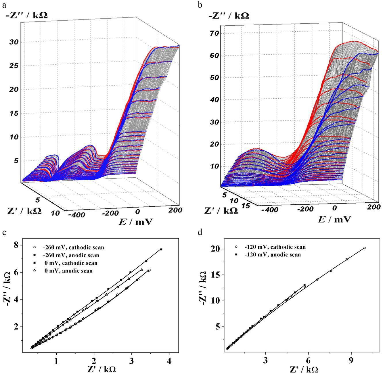
Fig. 1. Cyclic PDEIS spectra of (a) Pb upd on Au and (b) Pb upd on Au coated with selenium atomic layer; (c, d) examples of constant potential sections of PDEIS spectra for Pb upd on (c) bare Au and (d) Au coated with selenium atomic layer. Cathodic (red) and anodic (blue) scans in PDEIS spectra are presented in different colours in the electronic version.  $dE/dt = 2 \text{ mV/s}$ . Solid lines in (c) and (d) show fit to corresponding equivalent circuits.
